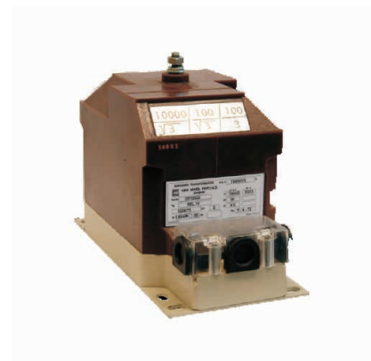
Voltage transformer 1-phase connection 12 or 24/110 kV class1, 50 VA;
